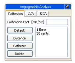
The calibration based on a known distance can be carried out by clicking the *Distance* button in the *Calibration* frame in the control. A list of names corresponding to the pre-set known distance values are shown in the white frame. Click with the left mouse button to select one.
