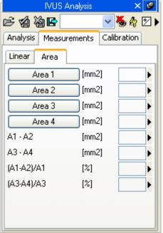
By clicking on the chosen button, the mouse pointer becomes a pen and with some simple clicks on the image, ComPACS traces the requested measurement.
