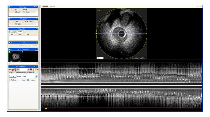
If the DICOM object is an IVUS sequence, you may perform a longitudinal reconstruction in real time during loop playback by clicking the *ILD* button. The position and the image dimension depend on the drop-down window near the *ILD* button.
