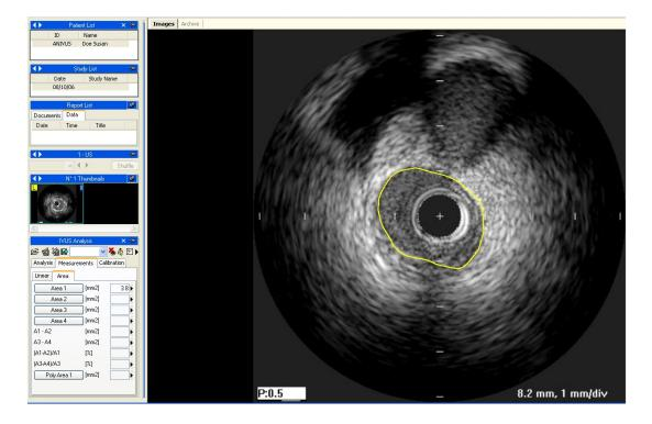
In case of angle measurements, the system automatically uses the center of the image as a reference point. It is therefore sufficient to click two points, moving clockwise, to measure an angle. In case of errors, you may delete a point using the right mouse button or, with a double click, entirely cancel the measurement.
