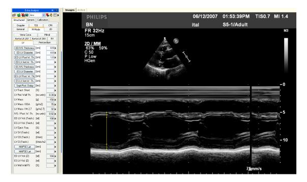
Not all the measurements are available on all types of images. For instance trying to perform a 2D area measurement on a Doppler image produces an error; in fact Doppler is not calibrated to make 2D area or length measurements. Or vice versa, if you try to measure a velocity on a 2D image, the software will again display an error message.
