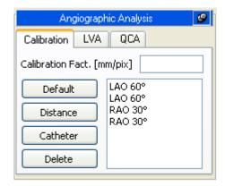
Default calibration can be carried out by clicking the *Default* button in the *Calibration* frame on the control window. In the white frame a list of names corresponding to the pre-set default calibration values are shown. Click with the left mouse button to select one. The corresponding calibration value will be displayed in the dedicated edit box above.
